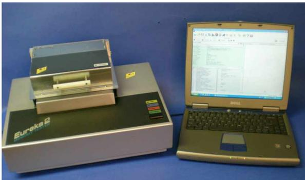
The CST new "ABT" Heat Chamber **Box System** provides a unique and cost-effective approach to testing memory modules up to 80 Degree C. This compact system is ideal for "bench top" applications and includes an integrated thermal heater box using – Halogen Lamp technology for rapid heat ramp-up and precision temperature control for Heat and Cool down.
